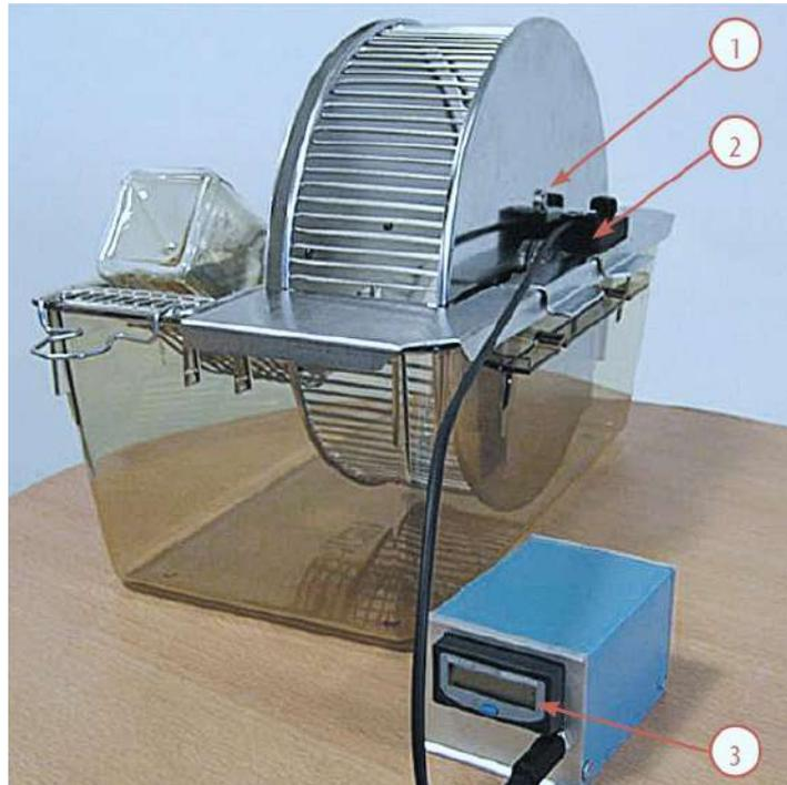
\* The magnetic switch counts the revolutions of the activity wheel according to the number of magnets mounted on the wheel:
